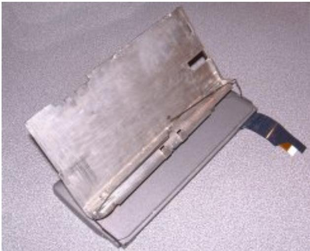
Now open the screen and keep going so it goes right past the battery compartment and almost under the chassis. Take care to ensure the flexi slides nicely through and then out of the chassis slot. This allows access to remove the springs
