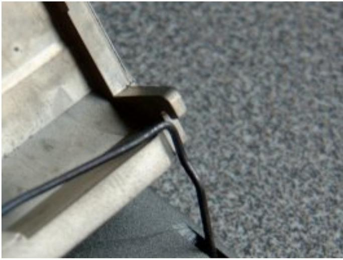
Now slide the screen slightly to the left and then to the right to release the springs from the side clips and hence the screen from the chassis.
